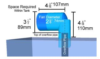
The Fan intake is designed to extend into the water, which creates a seal between the fan and the over flow pipe:
